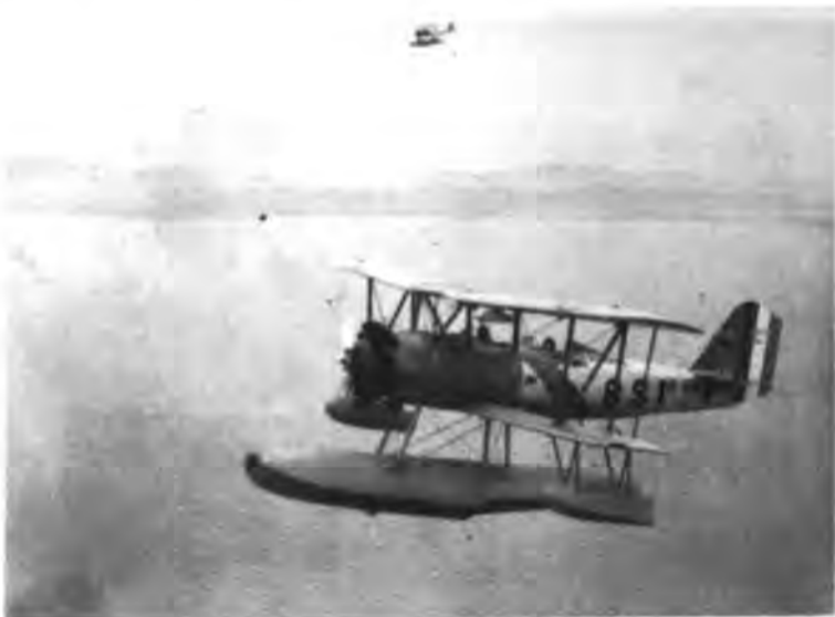
Vought Scout Plane flying near Manila, P.I. 1931. Note generator mounted on top wing
